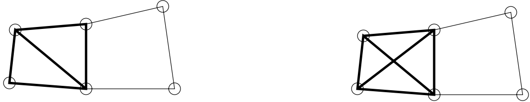
Figure 1.1: On the left hand side: N_s = 6 sites, N_l = 8 links; the bold links form a rigid but not overconstrained cluster; the total number of degrees of freedom of the network is N_{flop} = 4 . Constraint counting is correct, as it gives N_{flop} = 2N_s - N_l = 4 . On the right hand side: 6 sites, 9 links; the bold links form a rigid and overconstrained cluster; the total number of degrees of freedom of the network is still 4, since the added link is redundant. Constraint counting is not correct, as it would give N_{flop} = 3 .
