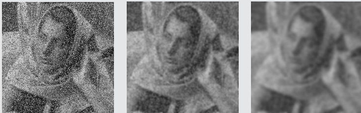
Figure 2 – (left) Impulse noise. (center) Gaussian filter \tau = 5 . (right) \tau = 11 .
