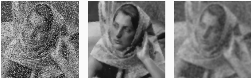
Figure 4 – (left) Impulse noise. (center) 9 \times 9 median filter. (right) Gaussian \tau = 4 .
