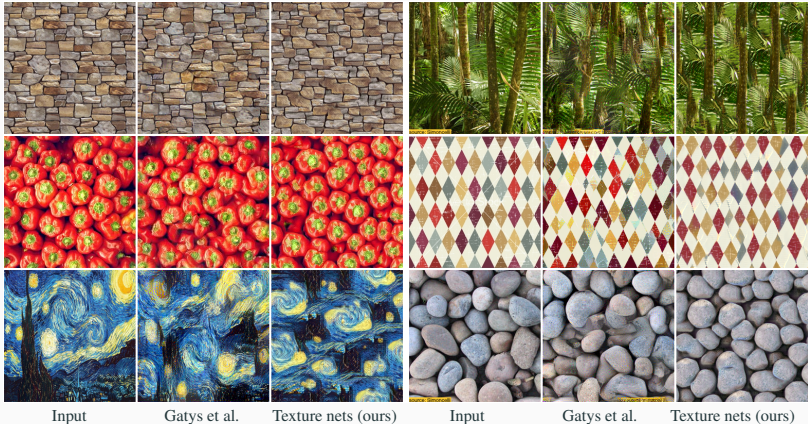
Figure 1. Texture networks proposed in this work are feed-forward architectures capable of learning to synthesize complex textures based on a single training example. The perceptual quality of the feed-forwardly generated textures is similar to the results of the closely related method suggested in (Gatys et al., 2015a), which use slow optimization process.
