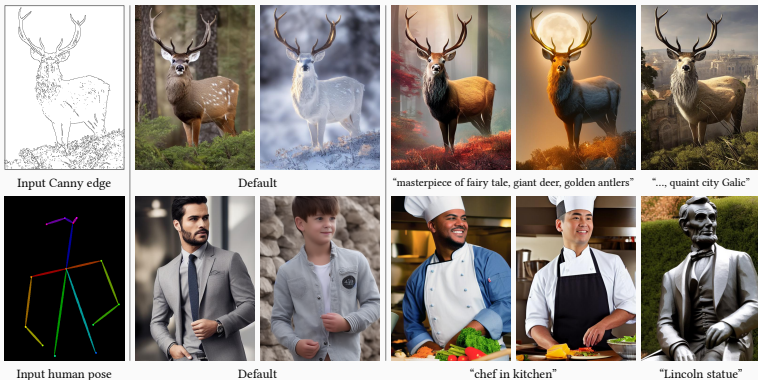
Figure 1: Controlling Stable Diffusion with learned conditions. ControlNet allows users to add conditions like Canny edges (top), human pose (bottom), etc. , to control the image generation of large pretrained diffusion models. The default results use the prompt “a high-quality, detailed, and professional image”. Users can optionally give prompts like the “chef in kitchen”.
